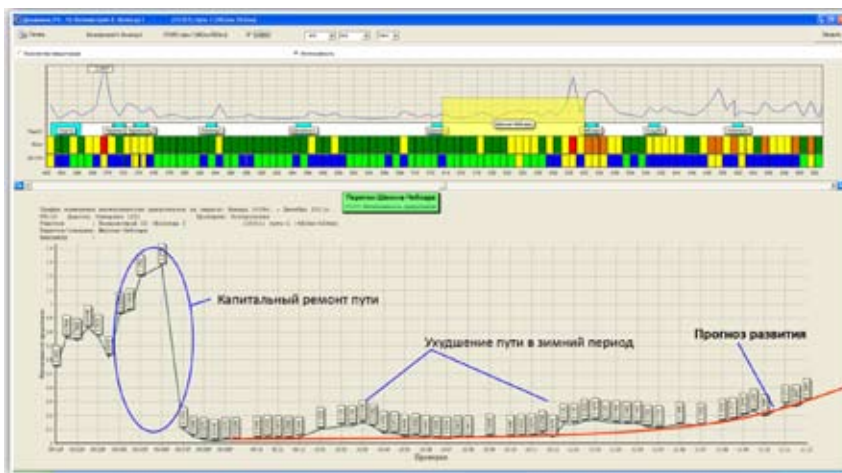
Figure 8: The dynamics of the development of the track state on a defined track section
