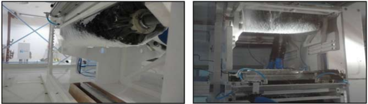
Figure 4. Electrospinning: Application of a wooden reservoir (left), and a glass reservoir (right)
