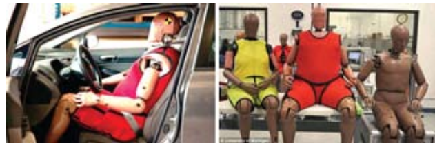
Fig. 5. (left) Photo of obese ATD ( \approx 124 kg), in the driving position and with a safety belt. (right) Comparative photo between ATDs of different sizes: on the left – “woman of 70 years”; in the centre – “obese man”; on the right – “standard man”. Image source (left): Splash News ( http://www.mirror.co.uk/news/weird-news/fat-crash-test-dummies-weigh-9812349 ). Image source (right): http://www.dailymail.co.uk/news/article-4212828/Crash-test-dummies-fatter-older.html .
