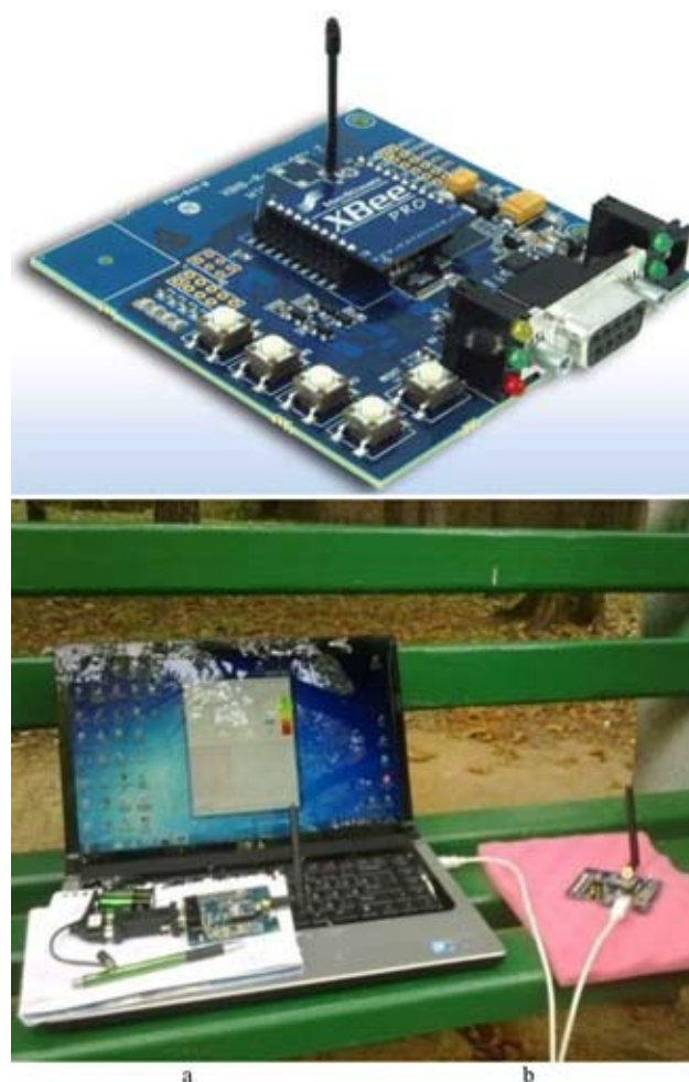
Fig. 1. Appearance of the Xbee (a) and set of equipment for the experiment (b)
